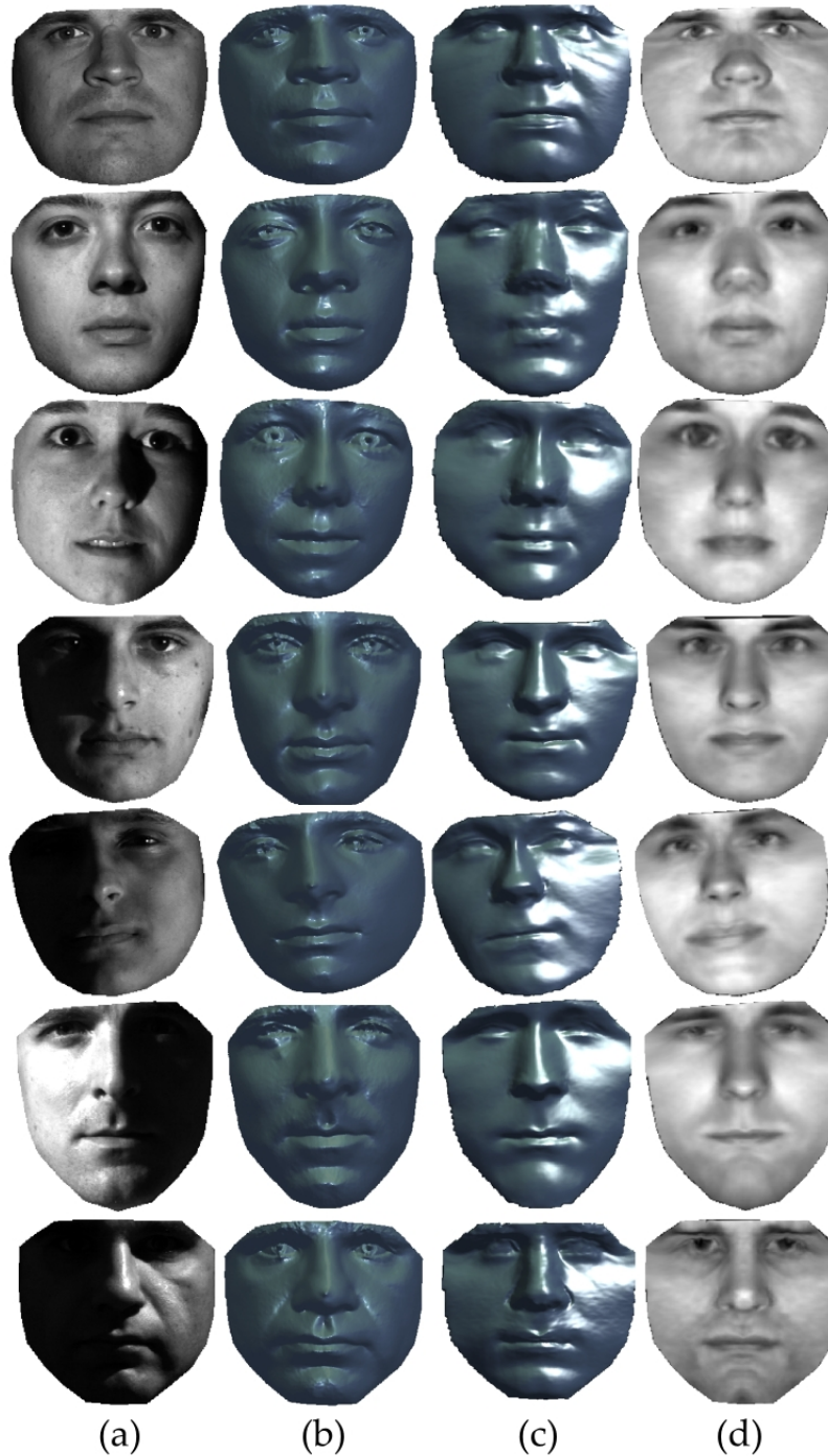
Figure 8.4: Recovered shapes for different YaleB Database subjects under same illumination conditions as in Figure 8.3, (a) Input image, (b) recovered shapes from photometric stereo using eight images from subsets 1 and 2 with known light directions, (c) recovered shapes and (d) recovered albedos.
